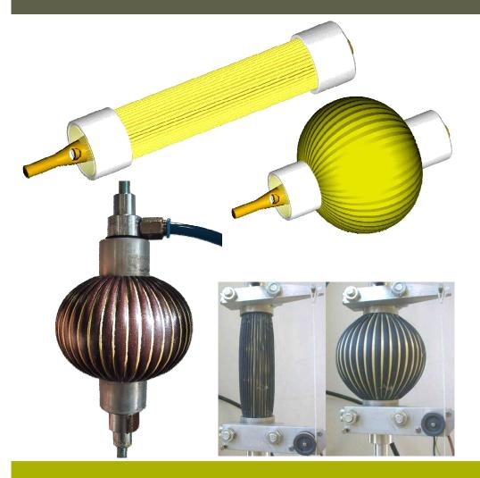
Pleated membrane Low weight (< 150 g!) High force levels Scalable No stick-slip No threshold pressure Direct joint attachment → No gear reduction, no backlash Inherent compliance
