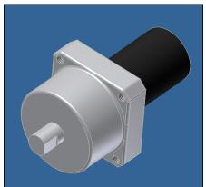
Fig. 70: CAD assembly of the motor (Maxon RE-40) and the harmonic drive (CSF Series Mini 5)
