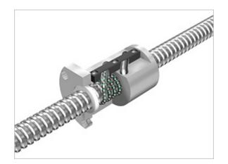
Fig. 59: Example of a ballscrew. Notice the tiny balls positioned between the nut and the screw. This will lead to a much higher efficiency than a conventional feed screw. This is a precision caged ball screw from THK. [16]
