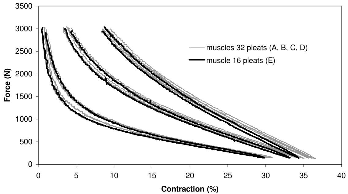
**Figure 3.26:** Measured forces as a function of contraction for five muscles at pressure levels 1, 2 and 3 bar
