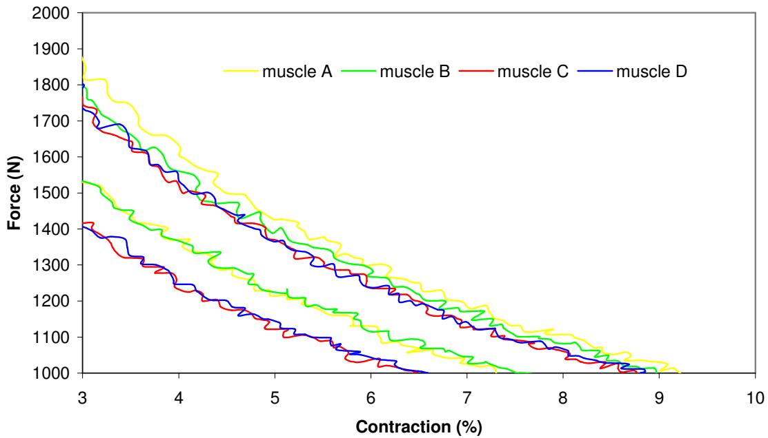
**Figure 3.24:** Detailed view of measured forces as a function of contraction for the four muscles made with 32 pleats at pressure level 1 bar
