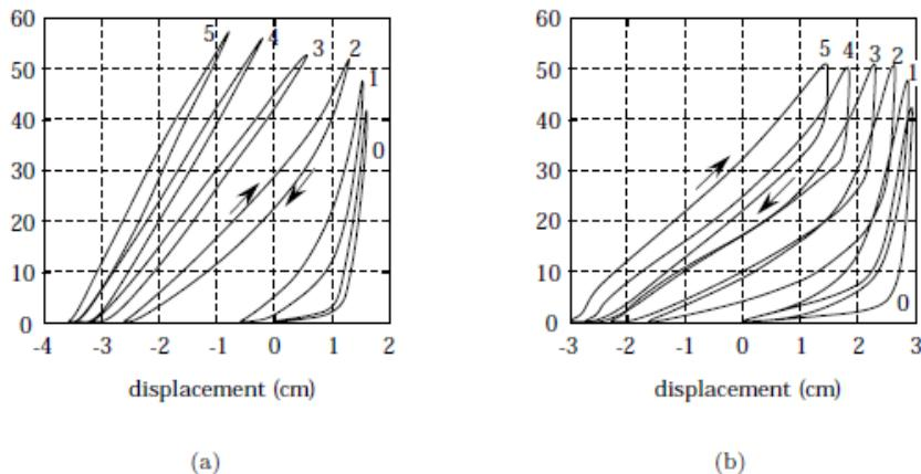
**Figure 2.7:** Mckibben Muscle tension (N) and hysteresis at isobaric conditions (0, 1, 2, 3, 4 and 5 bar), (a) Nylon braid, (b) fiberglass braid. [7]
