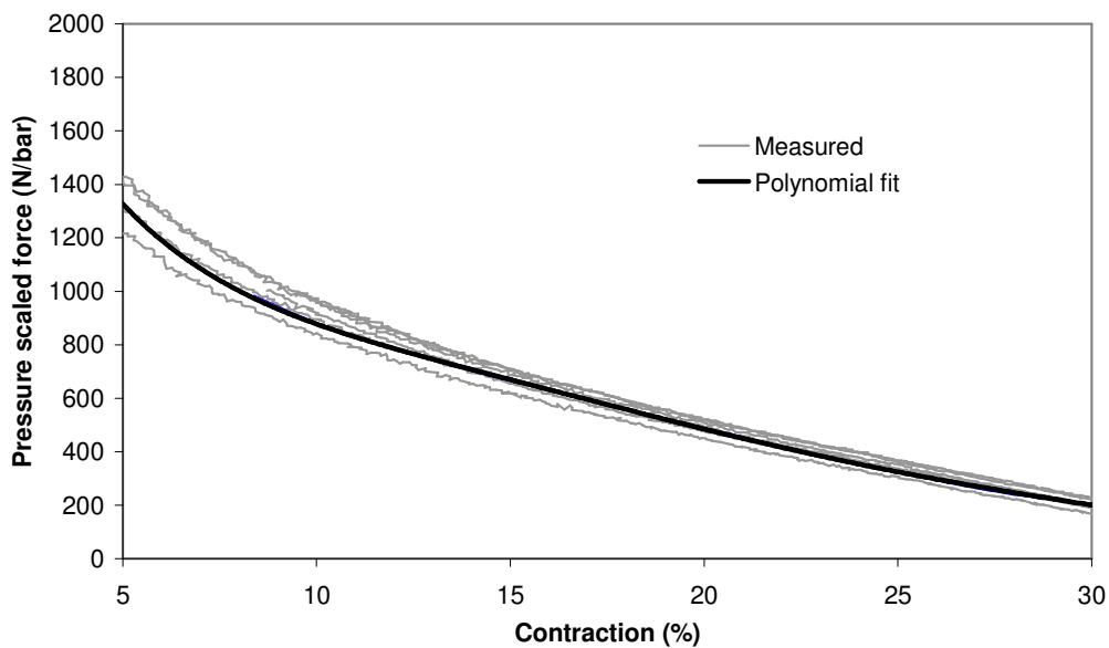
**Figure 3.30:** Pressure scaled measured forces as a function of contraction compared with polynomial fitted estimation for 1 muscle made with 32 pleats.
