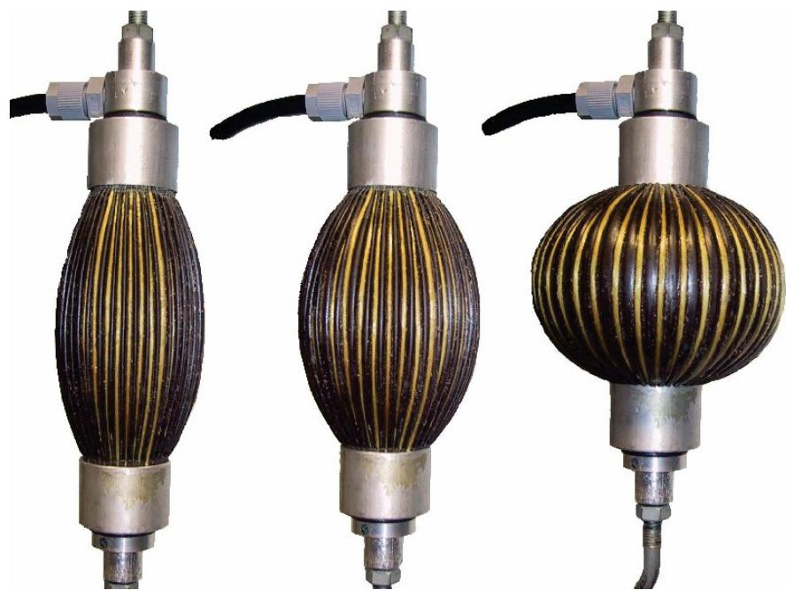
**Figure 3.5:** Photograph of three inflated states of the second generation PPAM
