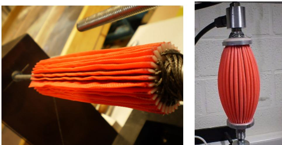
**Figure 3.12:** Photographs of the muscle prototype built with the plastic fabric
