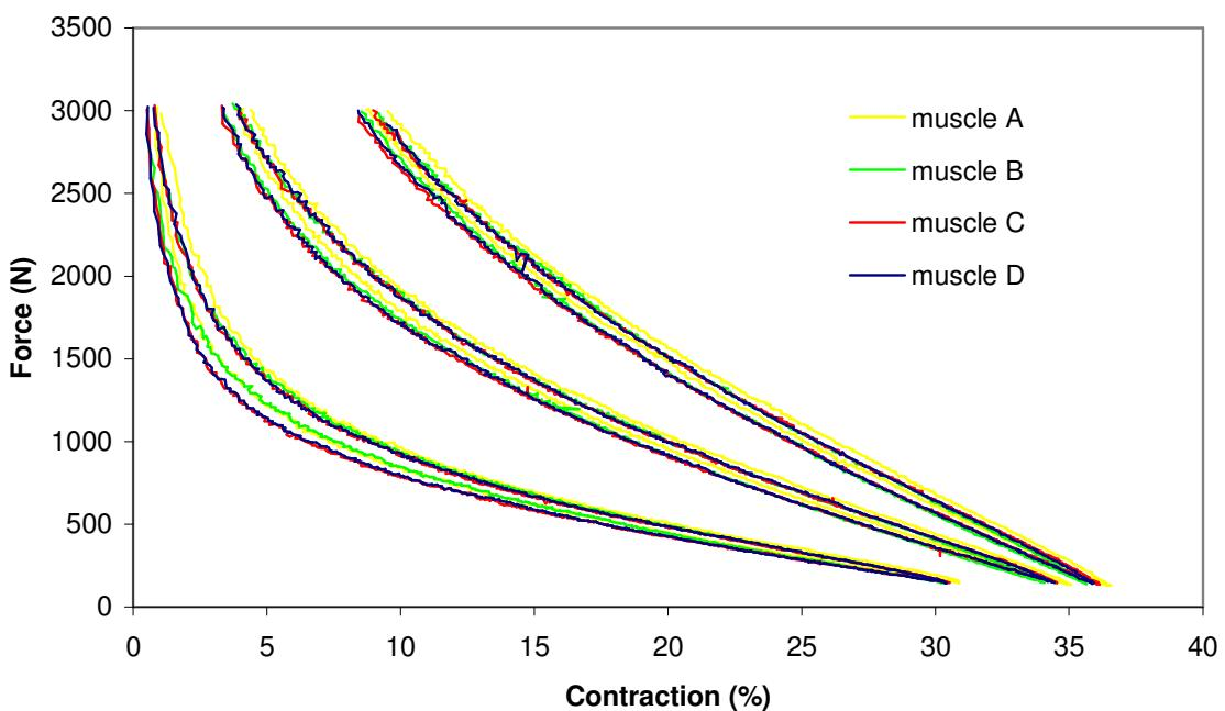
**Figure 3.23:** Measured forces as a function of contraction for the four muscles made with 32 pleats at pressure levels 1, 2 and 3 bar
