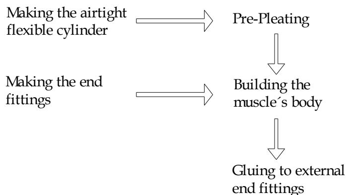
**Figure 3.18:** Diagram of the production process of the third generation of PPAM
