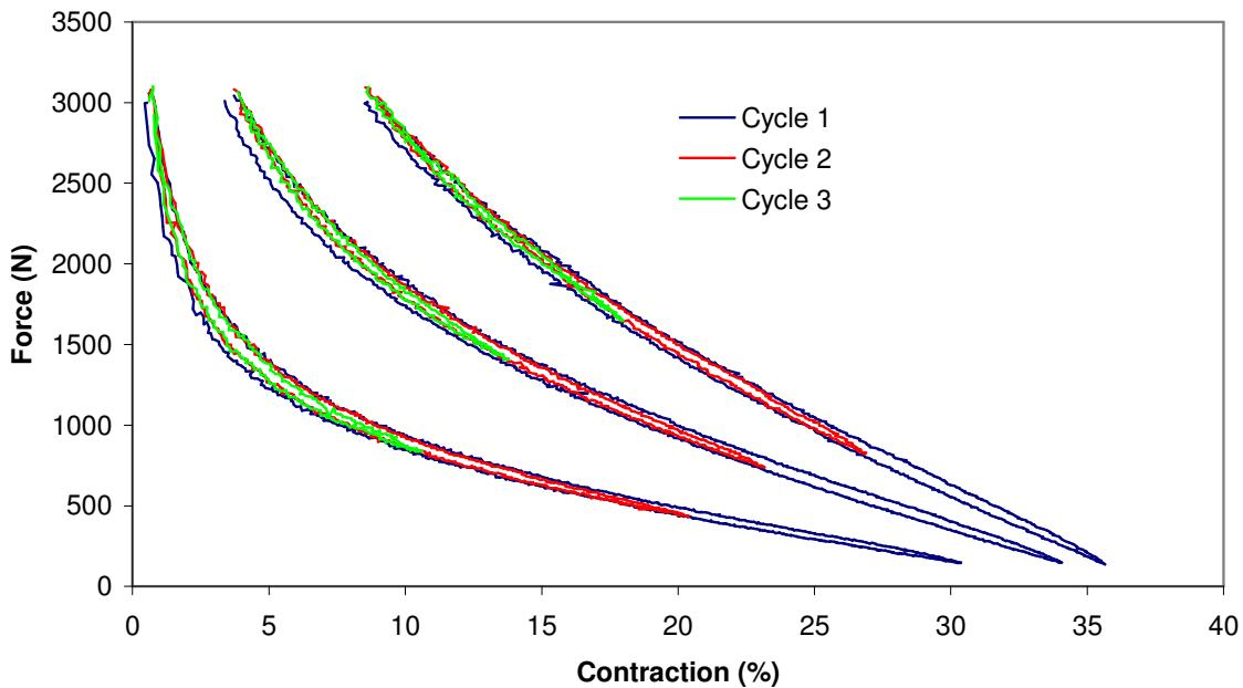
**Figure 3.25:** Measured forces during three cycles as a function of contraction for one of the muscles made with 32 pleats at pressure levels 1, 2 and 3 bar
