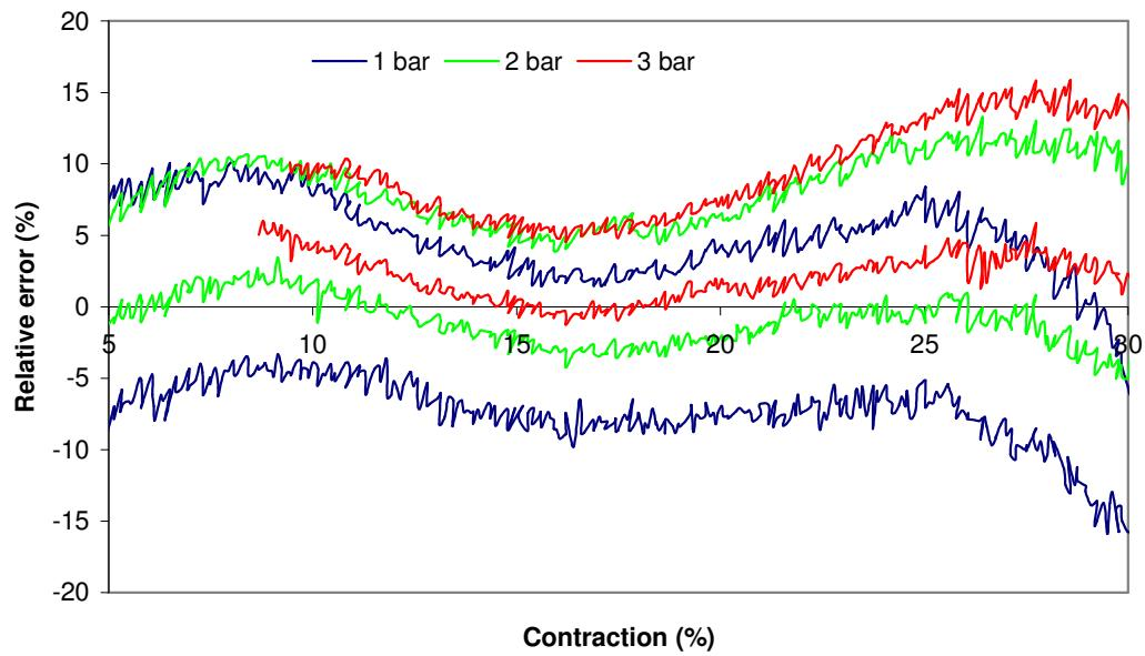
**Figure 3.31:** Relative error between the polynomial fitted estimation and the pressure scaled measured forces as a function of contraction for 1 muscle made with 32 pleats
