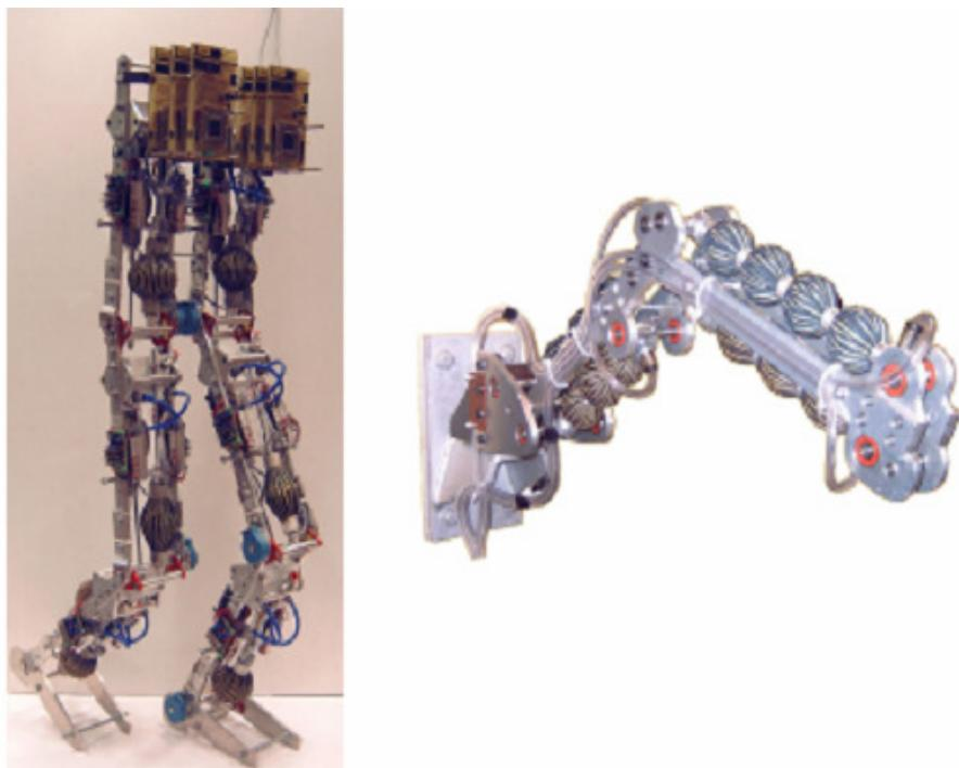
**Figure 1.1:** Photographs of Lucy (bipedal walking robot) and Soft Arm (robotic arm for direct human assistance) [3]
