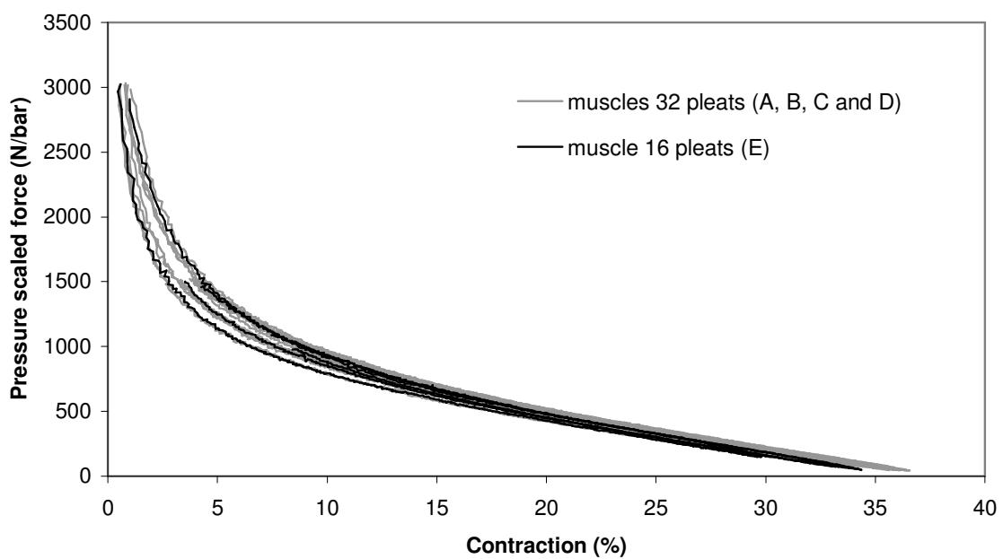
**Figure 3.27:** Pressure scaled forces as a function of contraction for five muscles
