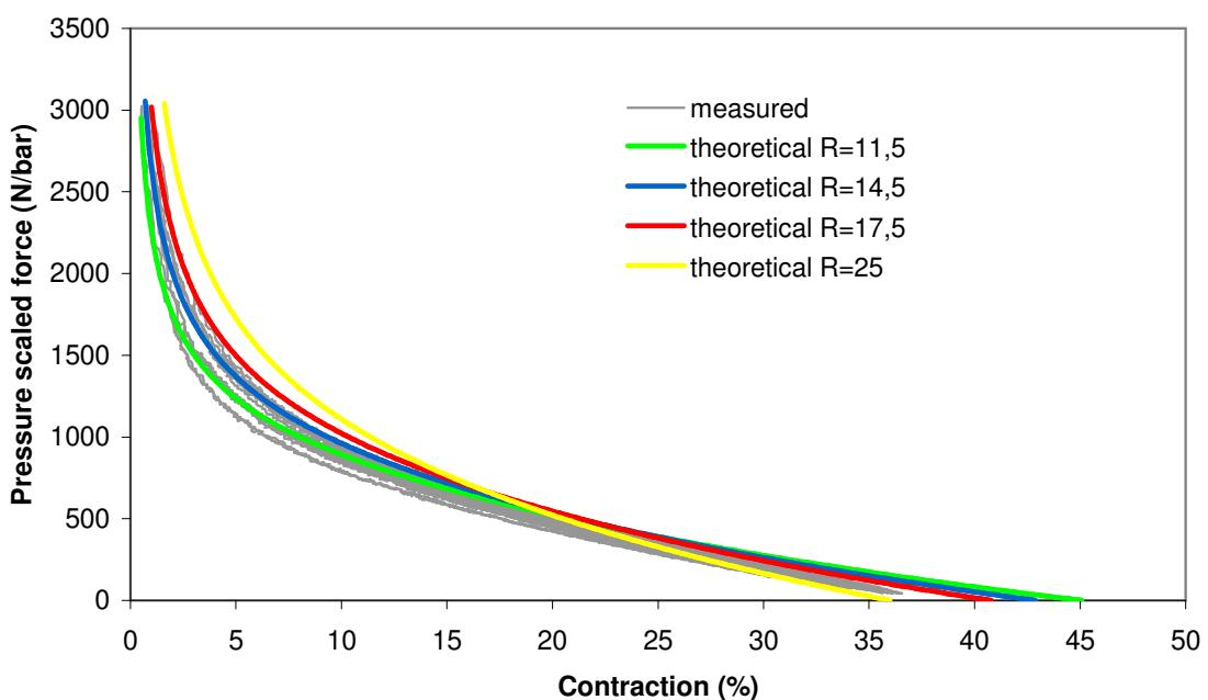
**Figure 3.28:** Pressure scaled measured forces as a function of contraction for 4 muscles made with 32 pleats compared with theoretical model
