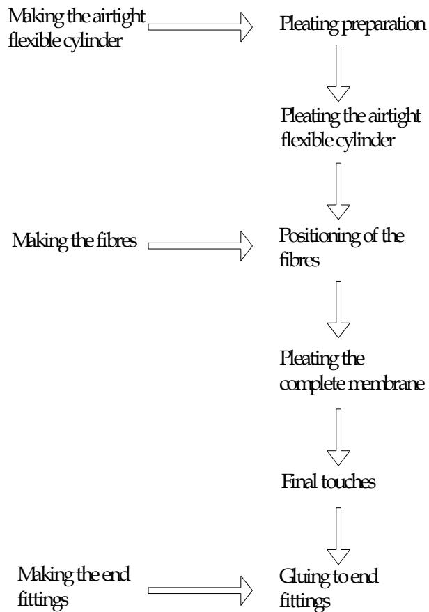
**Figure 3.6:** Diagram of the production process of the second generation of PPAM
