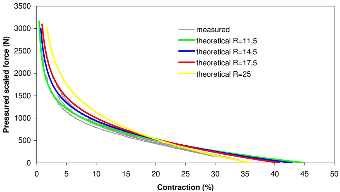
**Figure 3.29:** Pressure scaled measured forces as a function of contraction for 1 muscles made with 32 pleats comparedwith theoretical model
