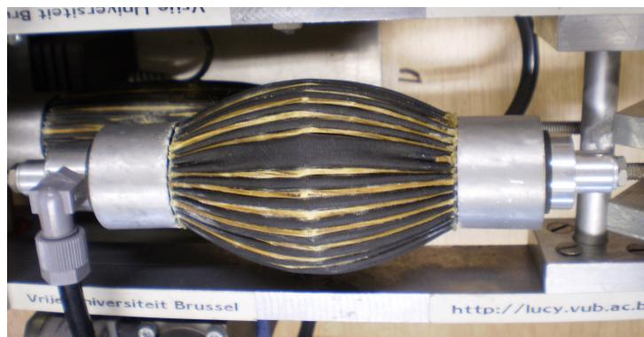
**Figure 3.9:** Photograph of a PPAM 2.0 with a broken fibre.
