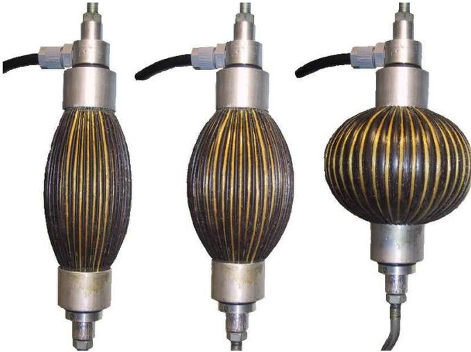
Figure 2.1: A second generation Pleated Pneumatic Artificial Muscle (PPAM) shown in three different values of contraction.
