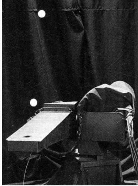
**Figure 1.4:** The spatial juggler—the “Bühgler Arm”—developed by Koditschek *et al.* which is capable of batting two balls simultaneously [59, 60]. This picture is taken from [8].
