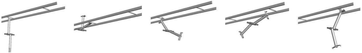
**Figure 6.10:** Pictures of the movement of the robot (simulation) when  $d = 1.3$ . 1. Initial state at  $t=0$ . 2. Swing phase at  $t=3.74$ . 3. Lift-off at  $t=6.35$ . 4. Flight phase at  $t=6.53$ . 5. Catching the next bar at  $t=6.69$
